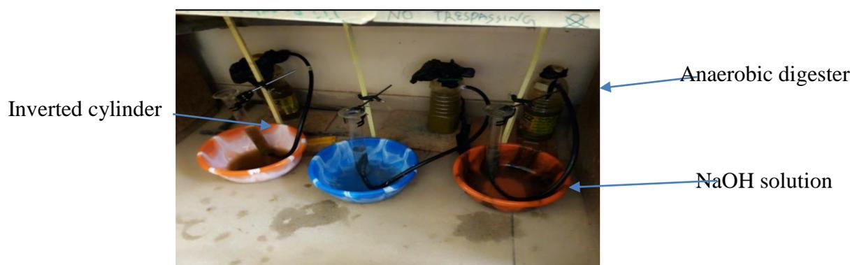
Plate I: Experimental set up for biogas production
