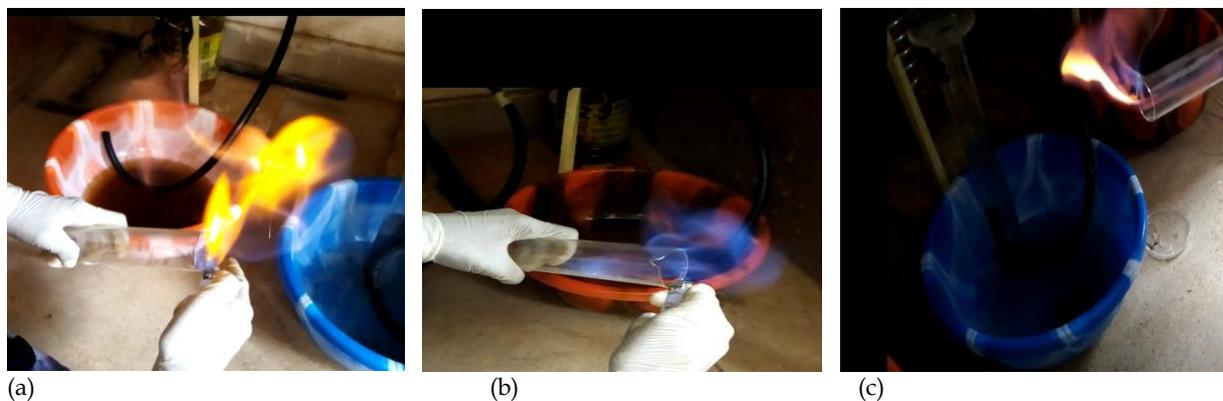
Plate II: Pictorial representation of flammability of biogas produced from the treated fruit waste
