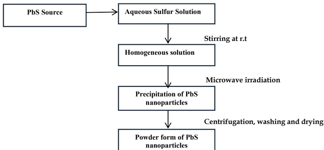
Figure 1. A schematic of the formation of PbS nanoparticles
