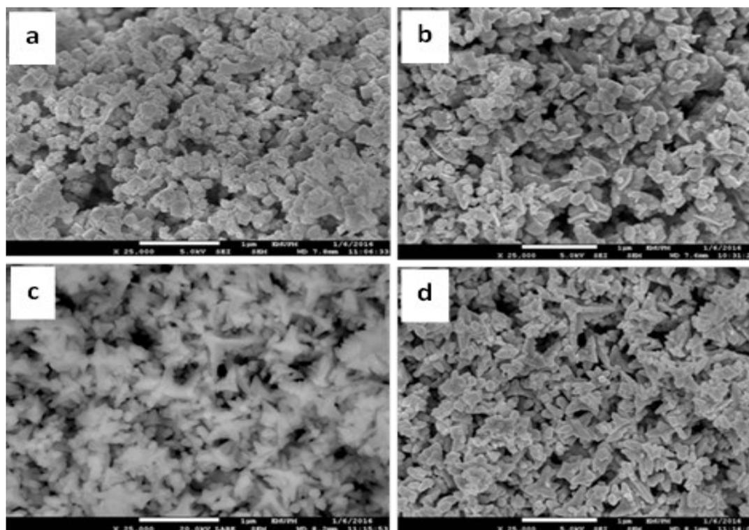
Figure 4. The FESEM Images of as-prepared PbS nanoparticles at different irradiation time: (a) 10 (b) 15 (c) 45 and (e) 50 min.
