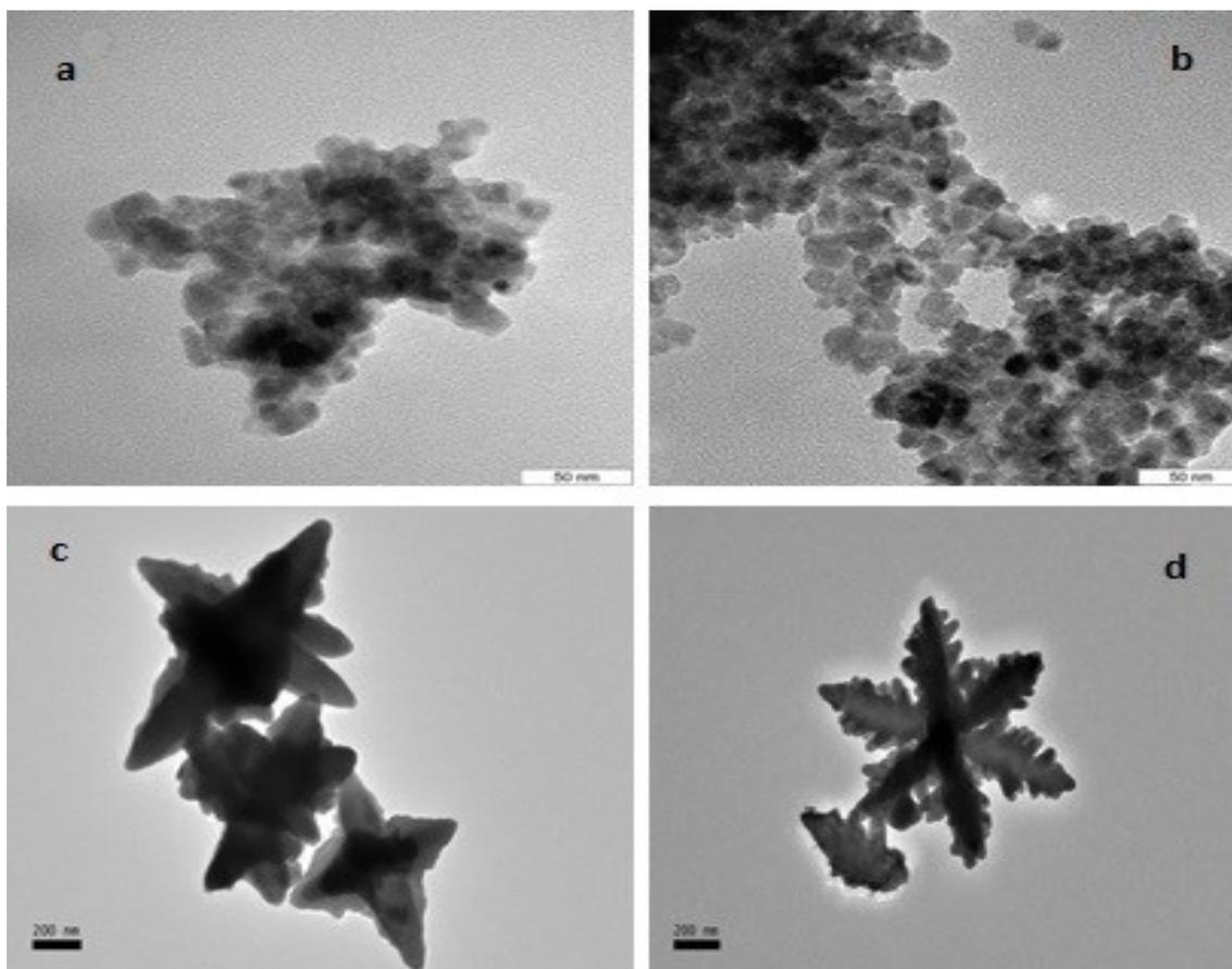
Figure 3. The TEM Images of as-prepared PbS nanoparticles at different irradiation time: (a) 10 (b) 15 (c) 20 and (e) 30 min
