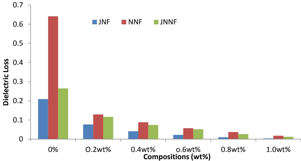
Figure 6: Dielectric Loss vs. Compositions of Titanium Oxide Nanoparticles.
