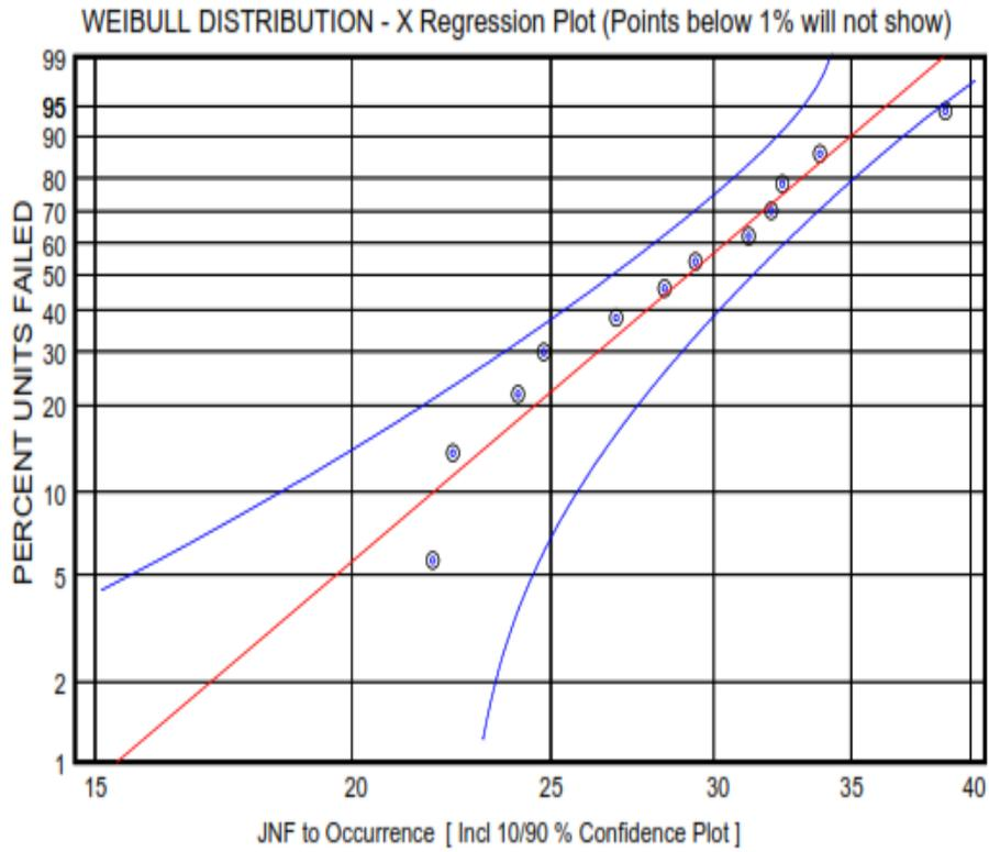
Figure 8: Weibull plot of Jatropha nanofluid (JNF)
