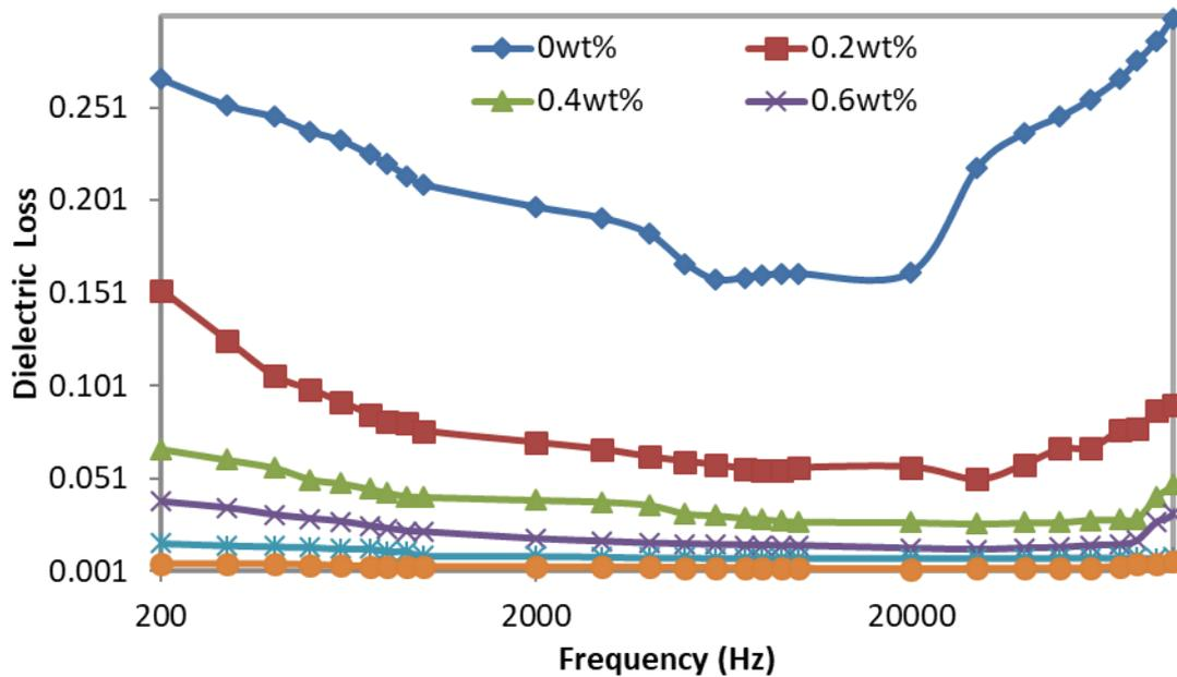
Figure 3: Dielectric Loss vs. Frequency (Hz) for Jatropha Nanofluid (JNF)
