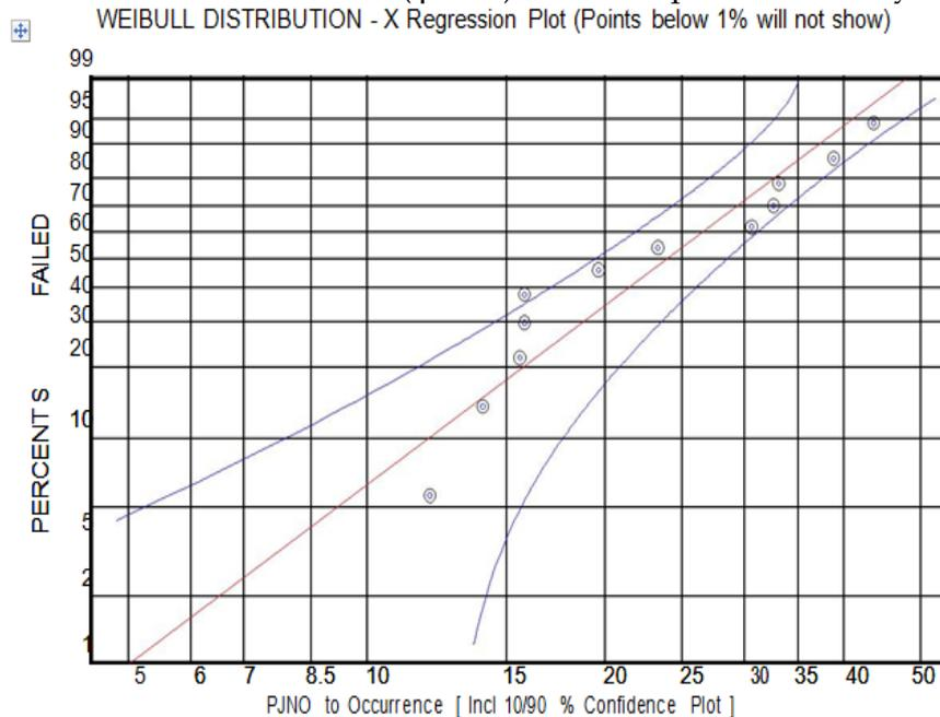
Figure 7: Weibull plot for Jatropha and Neem oil mixture (JNNF) Sample
