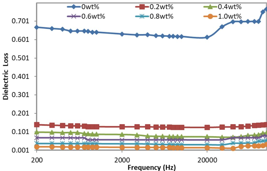
Figure 4: Dielectric Loss vs. Frequency (Hz) for Neem Nanofluid (NNF)
