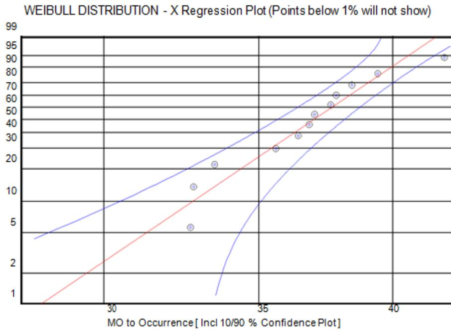
Figure 9: Weibull plot of AC breakdown field data for Mineral oil (MO)
