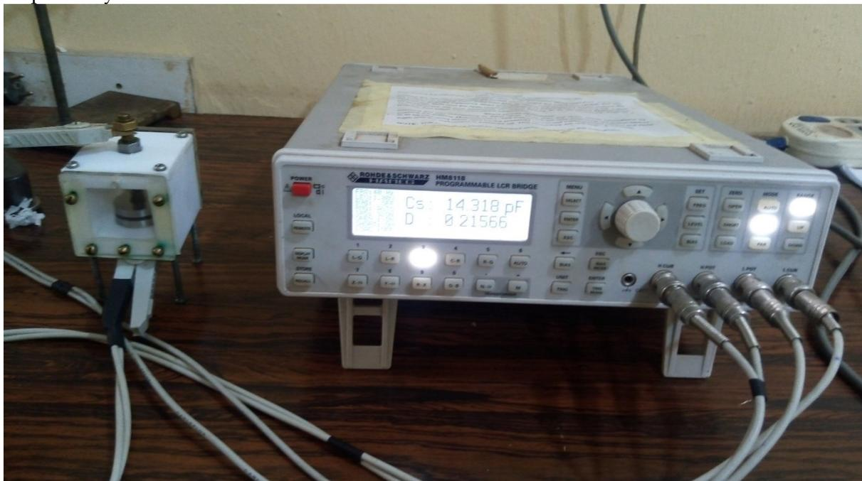
Figure 1: LCR Measurement of Dielectric loss
