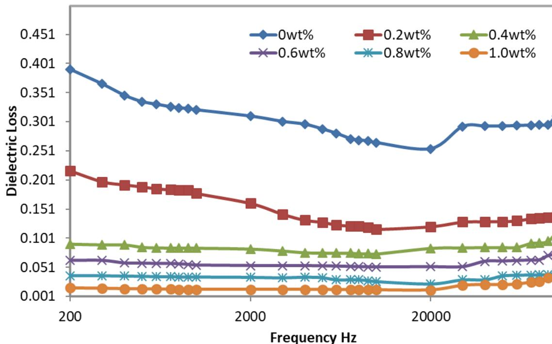
Figure 5: Dielectric Loss vs. Frequency (Hz) for Jatropha-Neem Nanofluid(JNNF)
