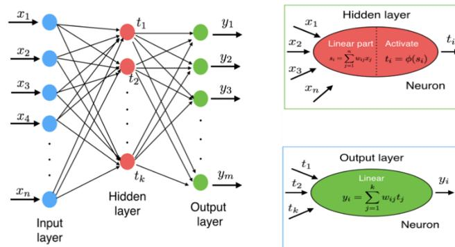
Fig. 1 A schematic diagram of typical three-layer ANN(Nasr *et al.*, 2012)
