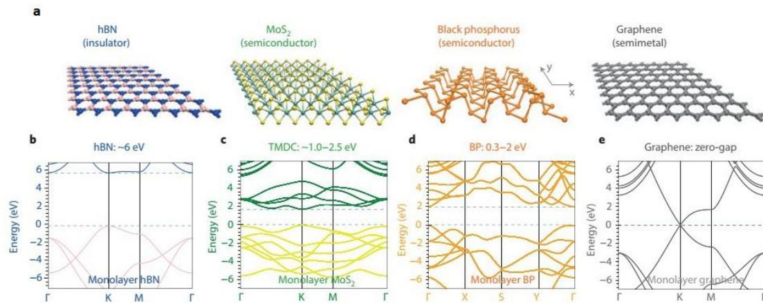
**Figure 1.** 2D materials covering a broad spectral range. (a) Structures and Band of single-layer (b)h-BN, (c)MoS<sub>2</sub>(d) BP and (e)graphene(Zeng *et al.*, 2018).
