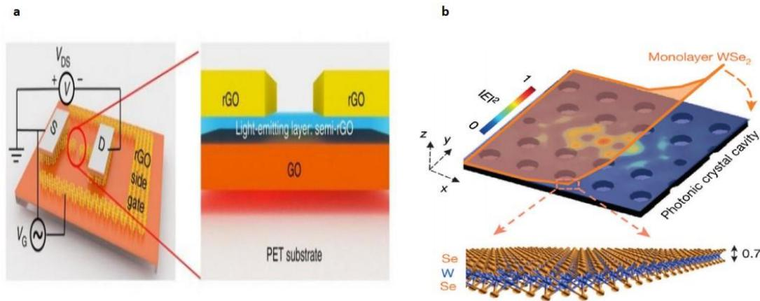
**Figure 3.** Schematic of (a) graphene-based field effect LED. A distinct semi-reduced graphene oxide (blue) at the interface between Graphene Oxide (orange) and reduce-graphene oxide (gold) is responsible for light emission (Wang *et al.* 2015). (b) Monolayer excitonic laser using WSe<sub>2</sub> on a PCC (inset scale bar 3  $\mu\text{m}$ ). Small mode volume and large overlap with the optical mode of the PCC contributed to the low lasing threshold (Wu *et al.* 2015).
