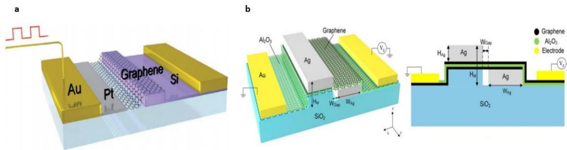
**Figure 4.** Schematic of: (a) First integrated graphene modulator using a doped silicon waveguide to gate the graphene layer. (b) 3D and cross-section of an electro-absorption graphene modulator integrated with a diagonal plasmonics waveguide.
