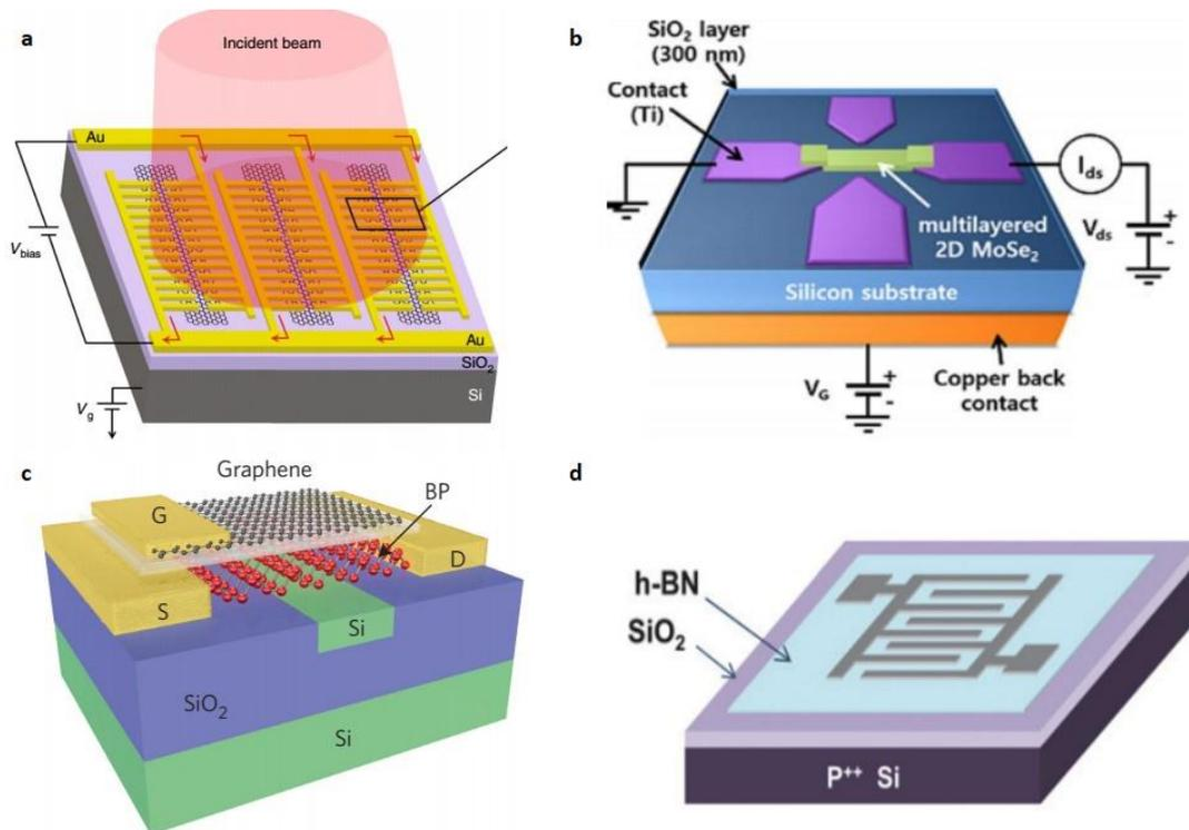
**Figure 2.** Schematic of: (a) a photodetector based on gold-patched graphene nano-stripes (Cakmakyapan *et al.* 2018). (b) High-performance near-infrared photodetector based on few-layered back-gated MoSe<sub>2</sub> (Ko *et al.* 2017) (c) BP device featuring a few-layer graphene top-gate (Nathan *et al.* 2016) (d) a h-BN photodetector (Liu *et al.* 2018).
