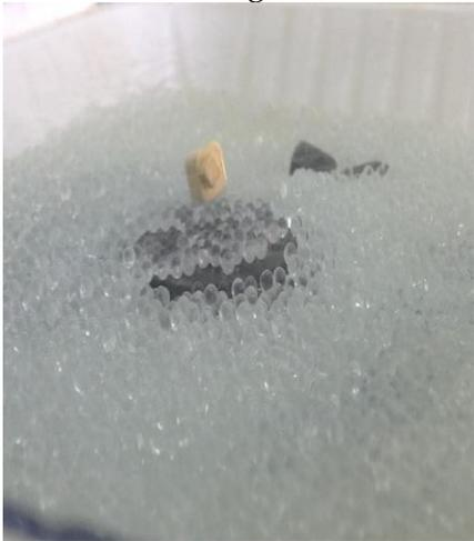
**Fig. 1:** A magnet levitating above a YBCO superconductor
