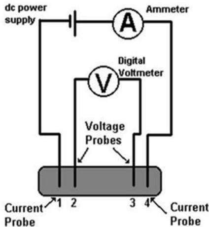
Fig. 3 Circuit diagram of Four-Point Probe [10]
