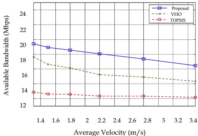
Fig. 3. Comparison of Available Bandwidth with Different MUE’s Velocities ( $c = 90$  dBm).
