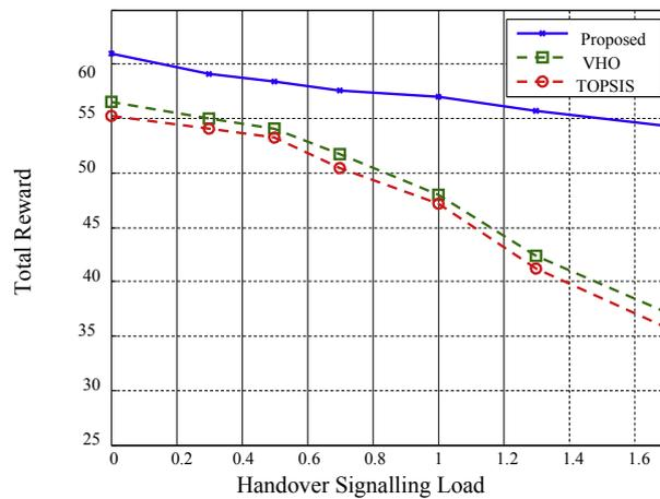
Fig. 6. Comparisons of Total Reward under different Handover Signaling Loads
