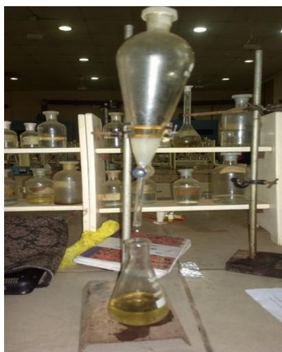
Figure 3. The glycerol layer remains in the separating funnel during the collection
