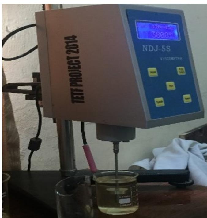
Figure 4. The digital viscometer used for measuring the viscosity of the biodiesel
