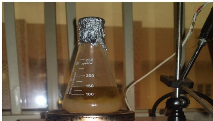
Figure 1. The ester layer at the top while the glycerol later at the bottom
