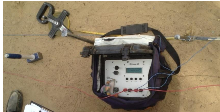
Figure 2:VES Survey Set Up
