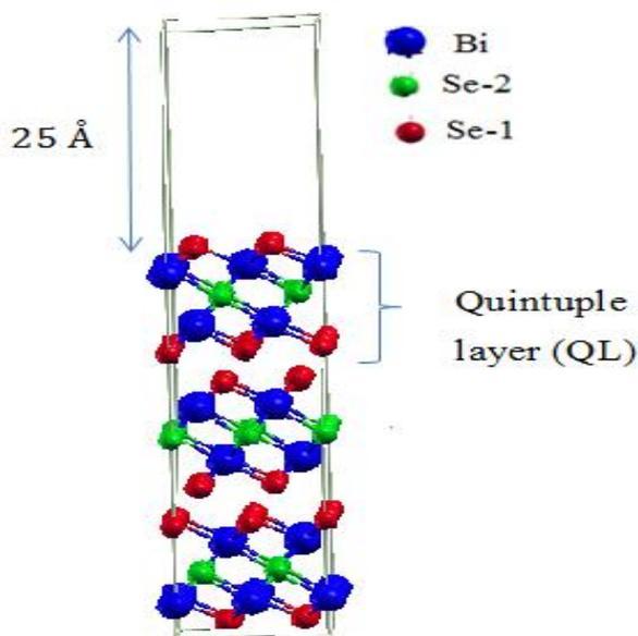
Fig. 1:(a) Crystallographic geometry of Bi<sub>2</sub>Se<sub>3</sub>
