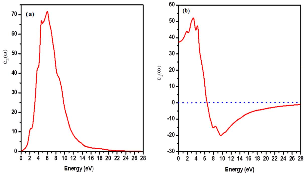
Fig. 4(a) imaginary part of the dielectric function (b) real part of the dielectric function of  $\text{Bi}_2\text{Se}_3$  surface states calculated using vdW-DF<sup>CO9x</sup>.
