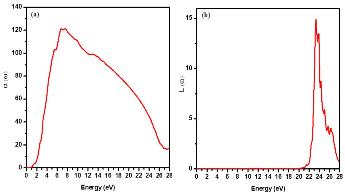
Fig. 5(a)Energy spectra of absorption coefficient  $\alpha(\omega)$ (b)EELS of  $\text{Bi}_2\text{Se}_3$  surface states calculated using vdW-DF<sup>CO9x</sup>.
