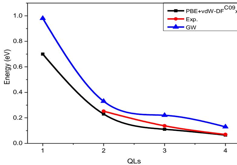
Fig. 3: Energy gap in function of film thickness for Bi<sub>2</sub>Se<sub>3</sub>
