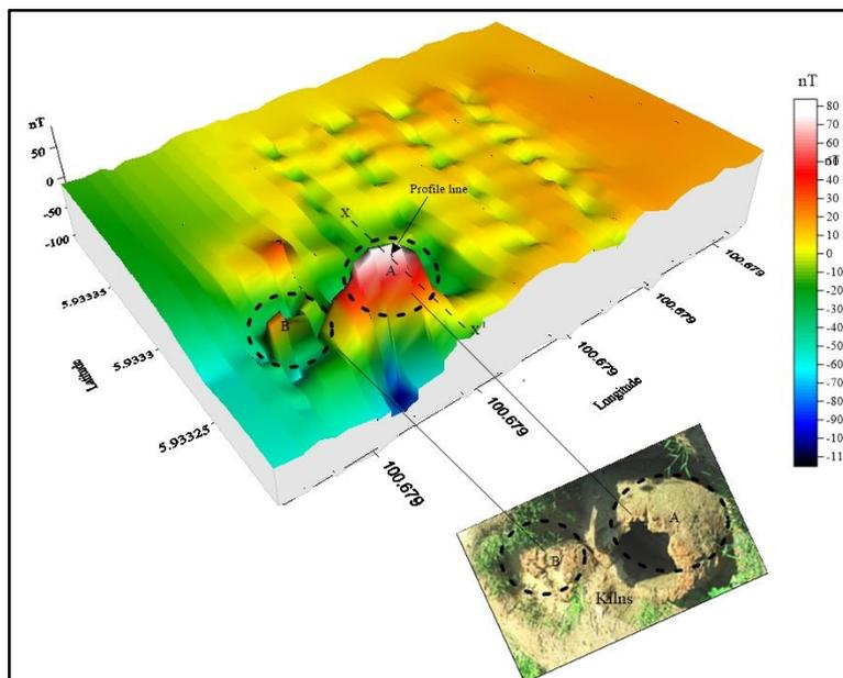
Figure 6: 3-D surface map of residual magnetic anomaly of the suspected target.
