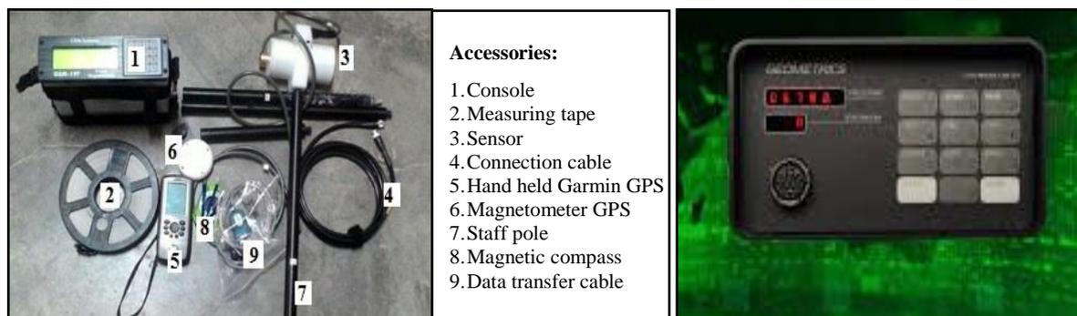
Figure 4: Magnetometer; (a) GEM system 19T and (b) G-856 console box
