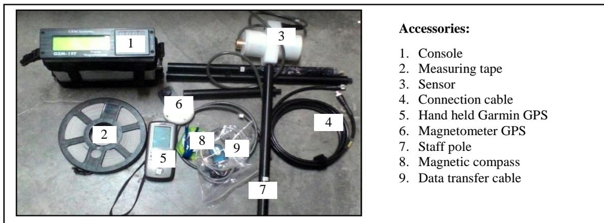
Figure 2: GEM 19T Magnetometer
