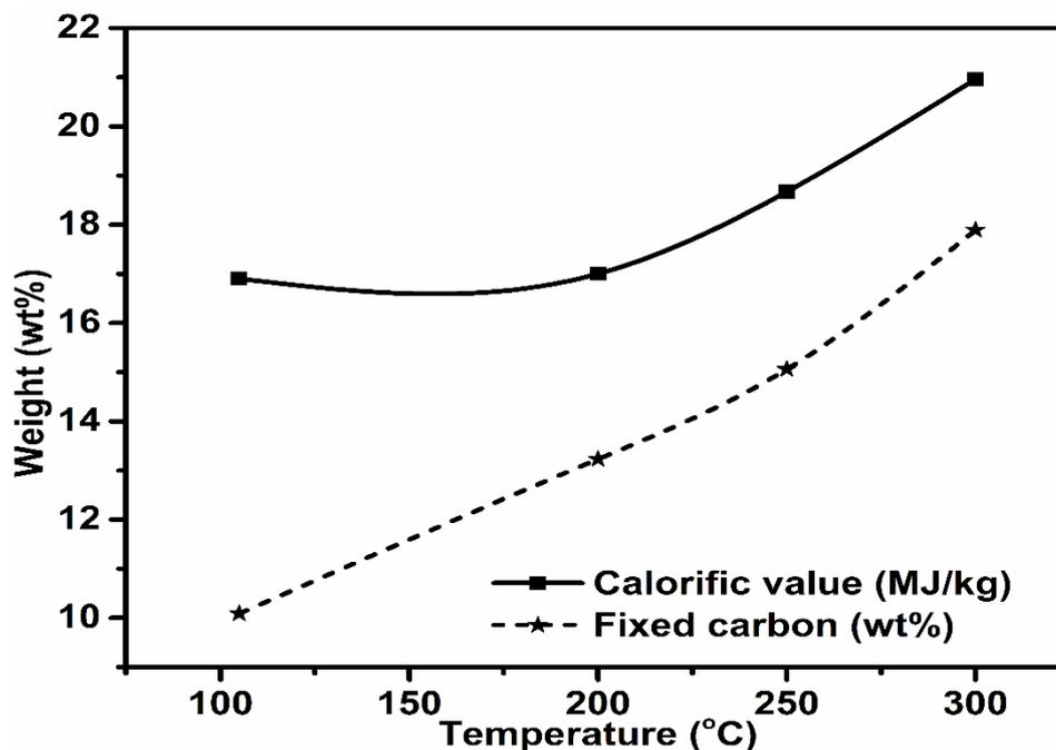
Figure 3: Increase in calorific value and fixed carbon versus temperature
