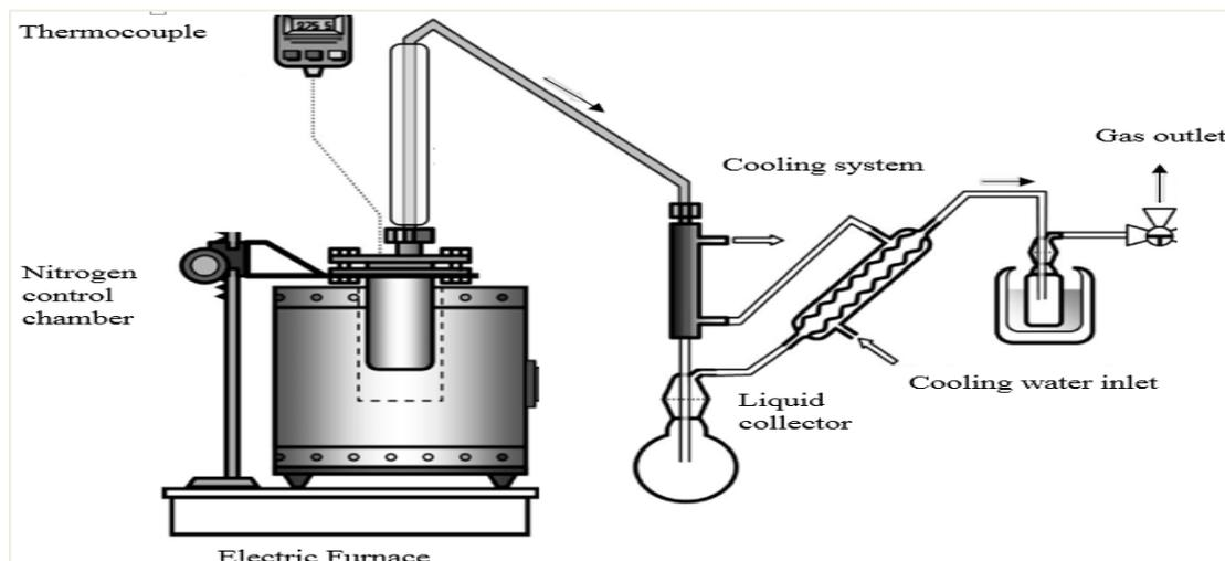
Figure 1. A schematic of the experimental system(Safana A.A et al. 2018).
