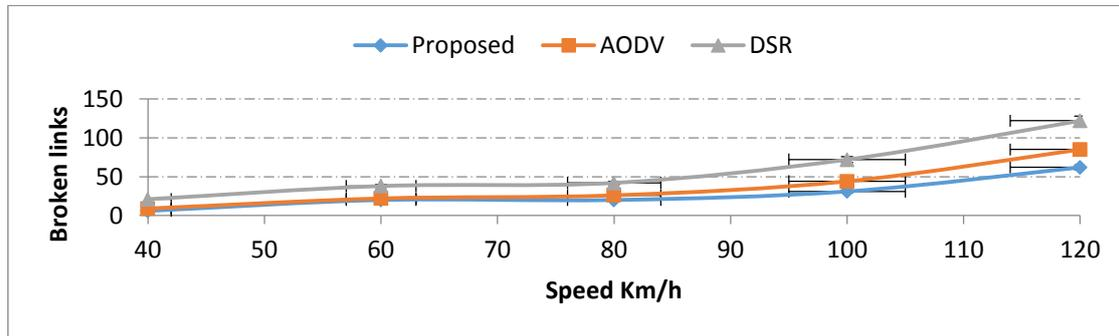
Figure 4: Number of Broken links with varying the speed of Vehicles
