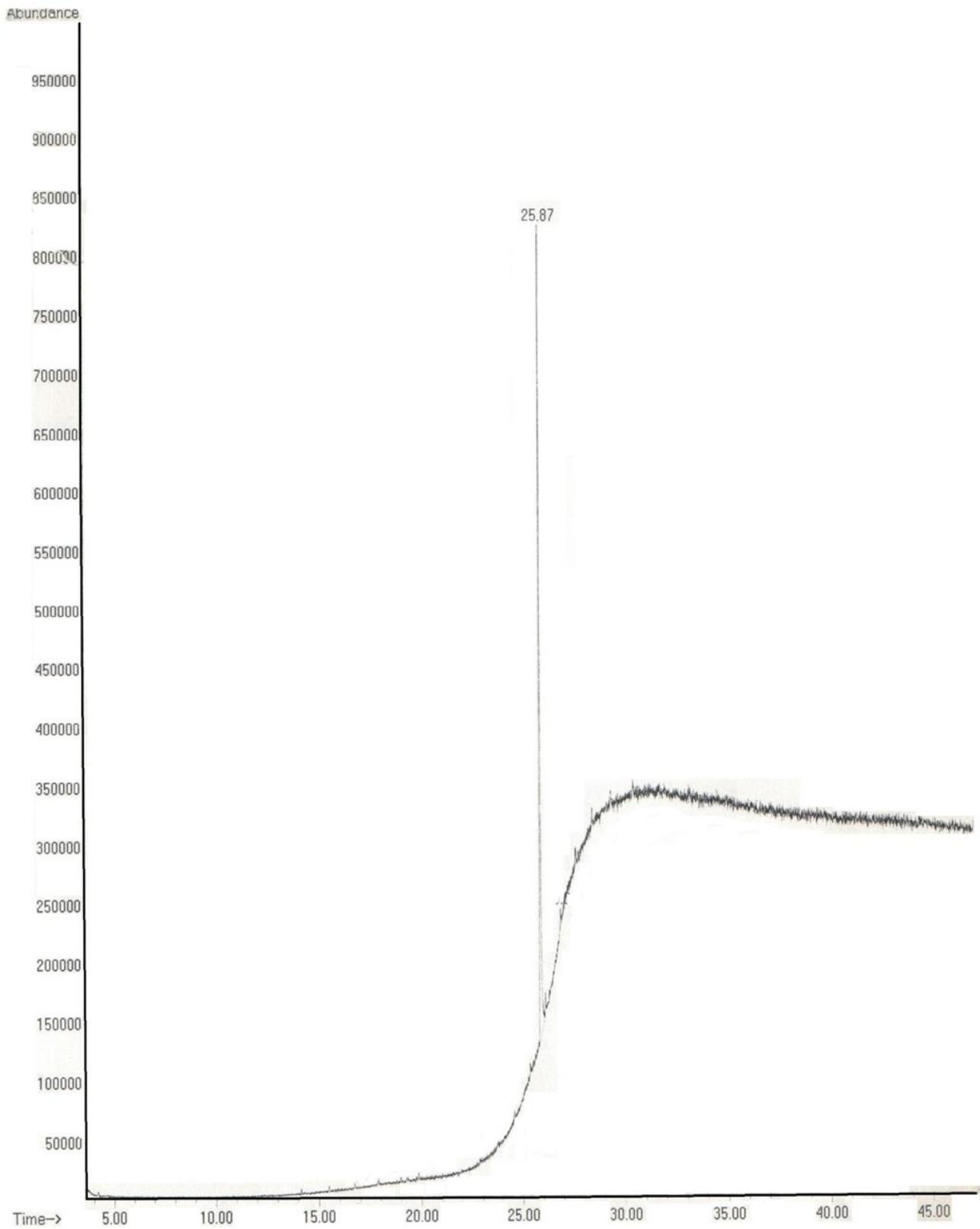
**Fig. 3: GC- Mass Profile of Essential Polyaromatic Oils in the Deasphalted Oils**
