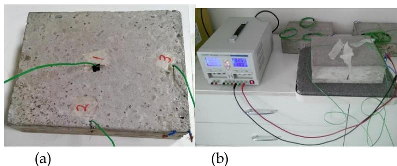
Fig. 2: (a) Thermocouples at three different locations and (b) carrying out experiment at room temperature
