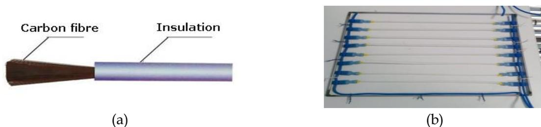
Fig. 1: (a) Continuous carbon fiber and (b) parallel arrangement of the fiber filaments as the heat panel
