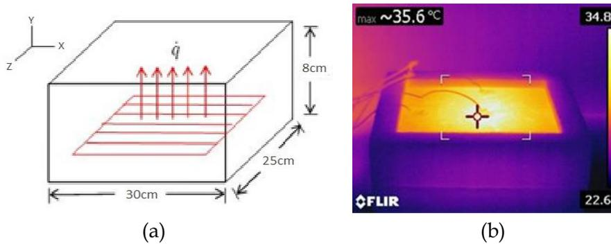
Fig. 3: Heat dissipated along the vertical direction (a) sketch and (b) IR image
