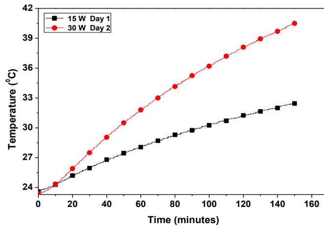
Fig. 6: Temperature variation with time for 15W/m<sup>2</sup> and 30W/m<sup>2</sup>
