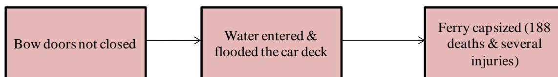
Figure 2: Hazard - Incident - Accident Chain
