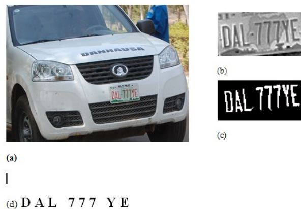
Figure 8: (a) Input image (b) Detected plate number (c) Segmented plate number (d) Recognized Character
